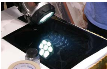
Shoeprint on mylar film lifted from newspaper with PathFinder
